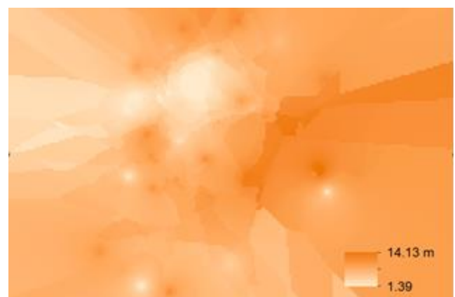
Fig. 3. The error field created by the interpolation of distance errors. The map extent is the same as Fig. 2.
