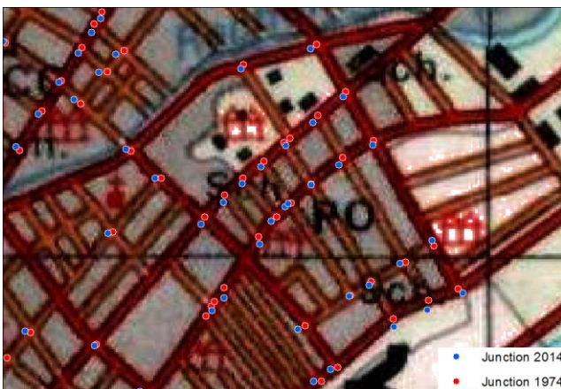
Fig. 2. Road network junctions for positional accuracy assessment. Red dots and blue dots represent the junctions digitalized from the 1974 paper map and extracted from the present authoritative spatial data respectively.
